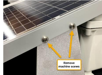
Figure 9: Remove the solar panel by removing these machine screws.
