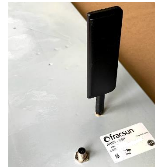
Figure 6: Blade antenna oriented straight and connected to SMA connector
