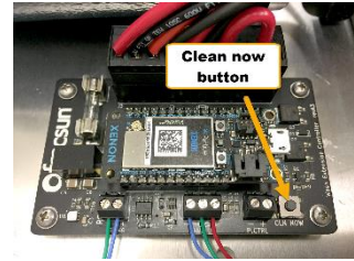
Figure 16: Manually test the pump with this button
